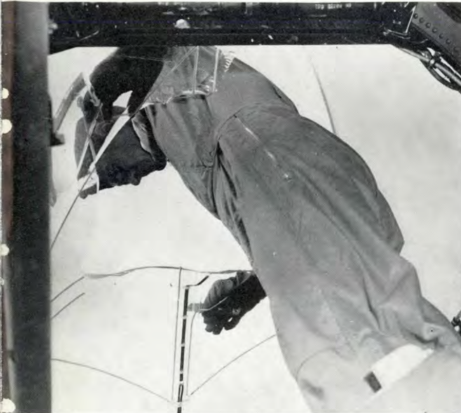
Pilot proves to himself on condemned F-101B canopy that you can bust out.
